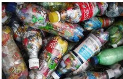
Some of our children are already making eco-bricks at home by stuffing mixed plastic waste into plastic bottles. A plastic bottle filled with plastic waste is very solid and can be used instead of regular bricks in construction. This technique is very simple and is suitable for many types of waste plastic. It is something we can do at Joy Lane too!
